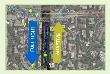
**Adaptive lighting** data were compared with two different conditions: full light and pre-programmed cycle regulation. Full light is the standard regulation for ROMA EUR lighting fixture. Furthermore, street lights were regulated measuring real time luminance and traffic flow, providing however correct luminance level as prescribed by UNI 11248.
